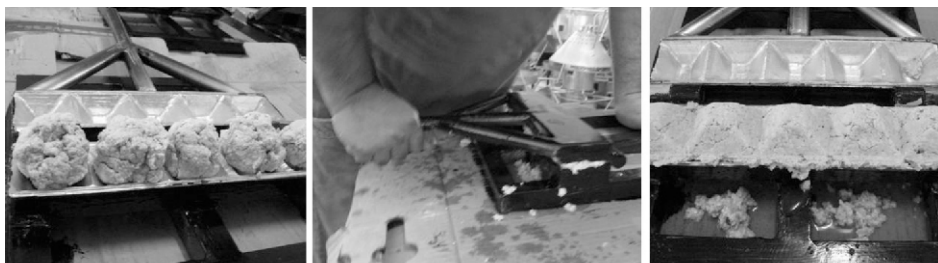
Figure 2. Briquetting of wastes, showing from left to right: placement of balled mixtures in the molder, compaction of the materials, and the pillow-shaped briquettes produced.
