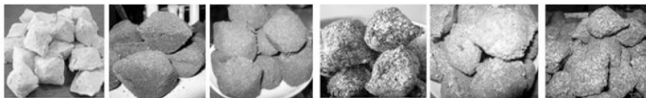
Figure 4. Types of briquettes produced using biomass and urban wastes, from left to right: paper, CRH, sawdust, paper and CRH, paper and sawdust, and paper, CRH and sawdust
