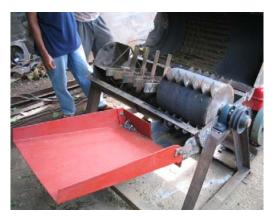
The small model of the machine can shred biomass material at a rate of 150 to 300 kg/hour, whereas the big model can shred 800 to 1000 kg/hour. The machine only requires 5-hp engine for the small unit and 17-hp engine for the big unit. Without the engine, the small unit costs P25,000.00 and the big unit costs P80,000.00. The cost of shredding biomass is P210.00 per ton of materials for the small unit and only P90.00 per ton of materials for the big unit.
