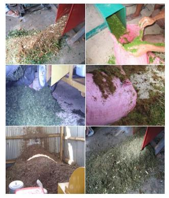
now possible because this technology applies the principle of cutting and beating actions of the knives and hammers in the shredding cylinder during the shredding process. The shredder can reduce the size of the biomass materials by 30 to 40% of its original size.
