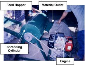
The machine basically consists of the following general assemblies: (a) the feed hopper, where biomass materials are held before feeding into the shredding cylinder; (b) the shredding cylinder, where the biomass materials are cut into smaller pieces and then beaten to rupture the fibers; (c) the material outlet, where the shredded biomass is discharged from the machine; and (d) the engine assembly, where the prime mover and transmission drive is located.
