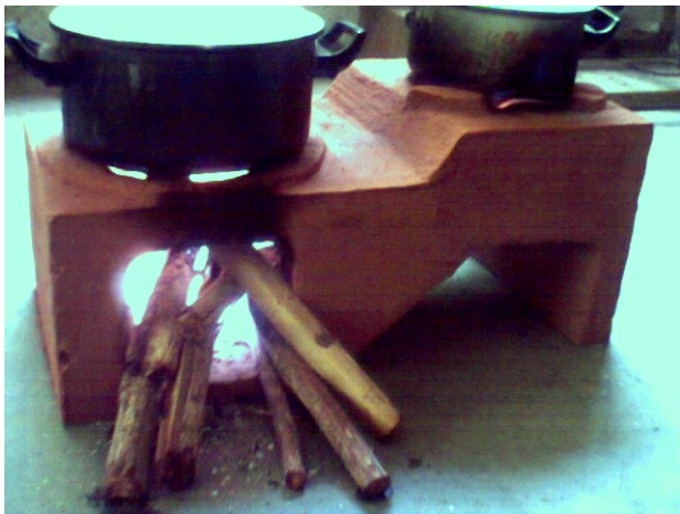
The Combustion Chamber
