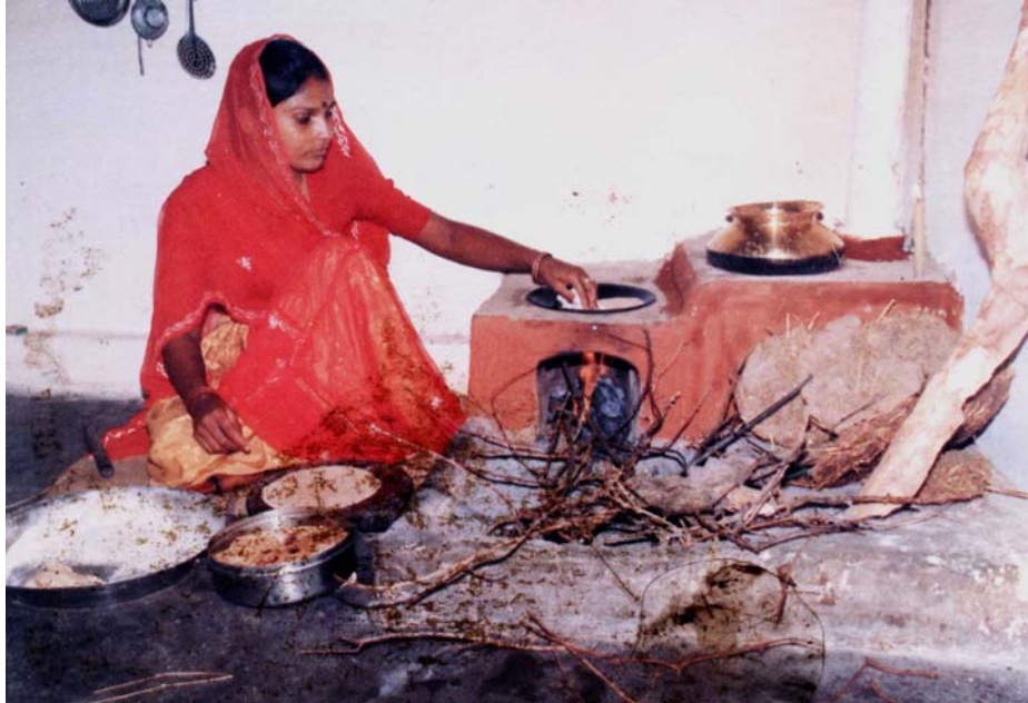
Double-Burner, Perpendicularly-Fired, and Chimneyless Stove
