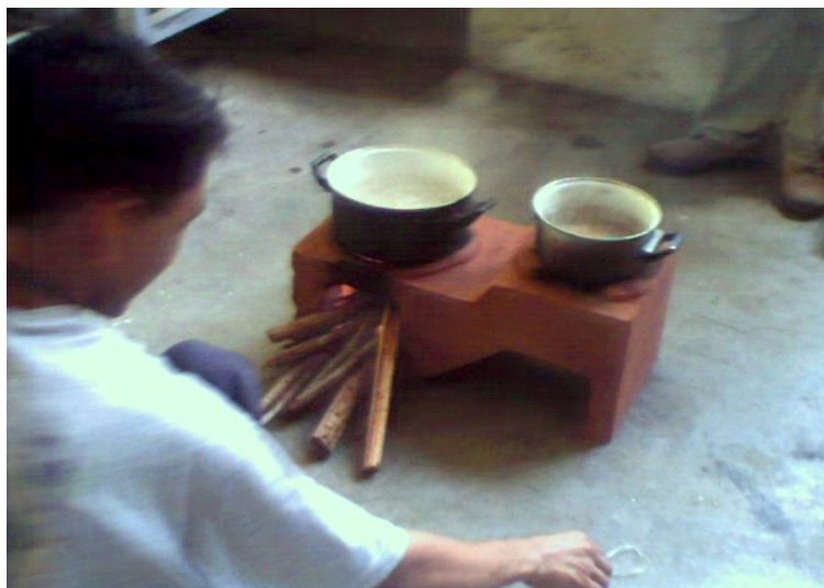
Figure 6. The Makini Stove During Testing.
