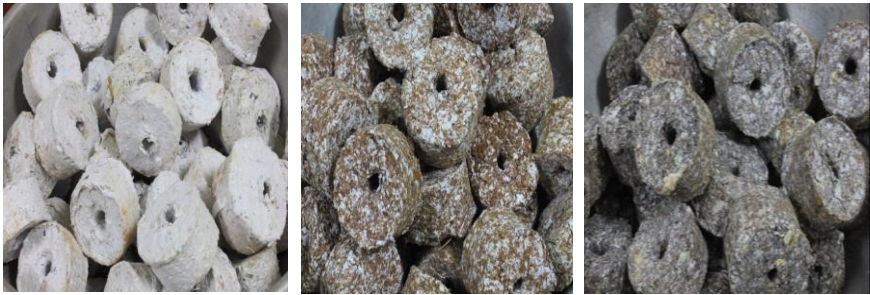
Figure 9. Types of briquettes produced using biomass and urban wastes, from left to right: paper, paper and sawdust and paper, sawdust and CRH.
