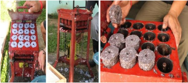
Figure 2. Briquetting of wastes showing “from left to right” the placement of mixtures in the molder, compaction of the materials, and removal of briquettes produced from the molders.
