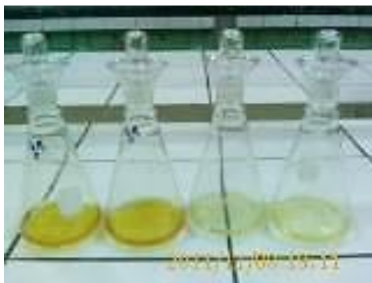
Figure 1. Color of the oil before and after heat treatments
