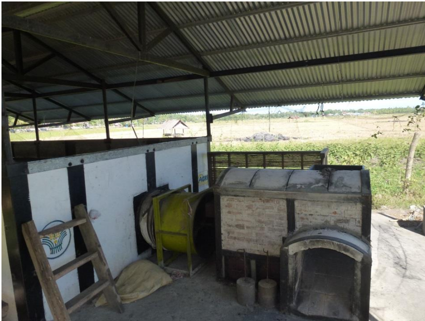
Figure 4-7: Flatbed dryer at an Irrigators Association in Brgy. Cansadan-Tubudan, San Jose, Antique
