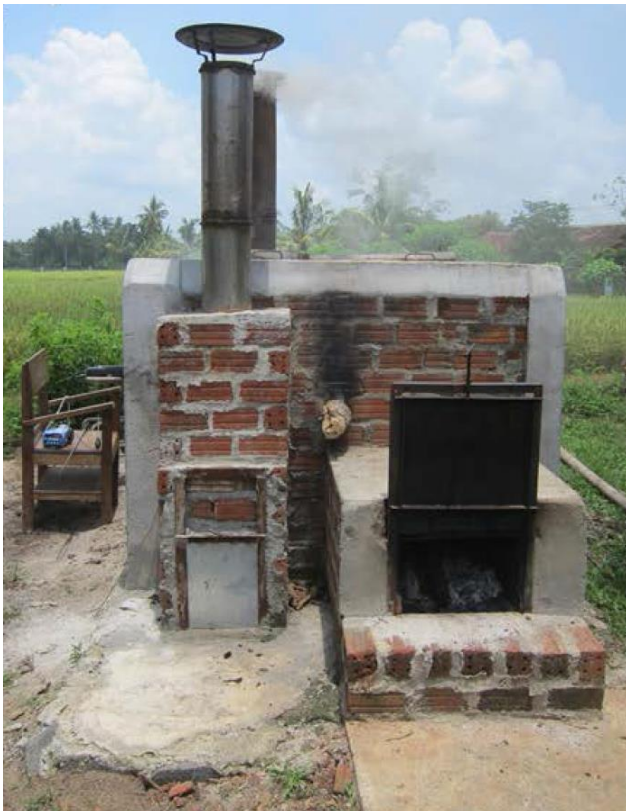
Figure 4-4: Adam retort in operation [9]
