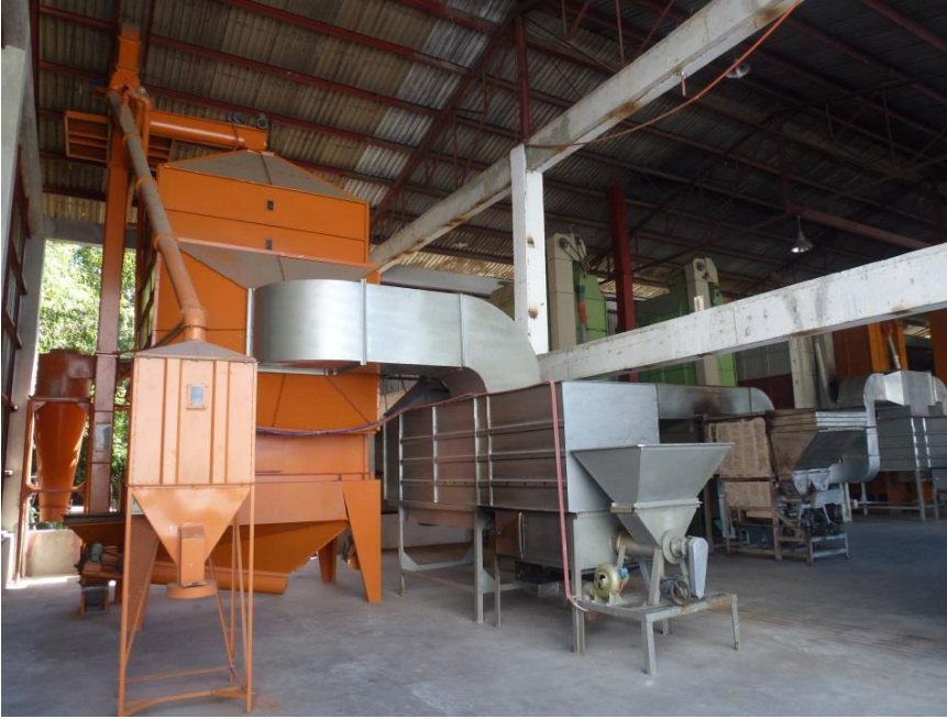
Figure 4-8: Circulating rice dryers at the National Food Authority (NFA) in Brgy. San Fernando, San José de Buenavista, Antique
