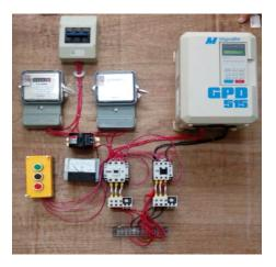
type motor load was controlled direct-on-line (DOL), the harmonics generated was about 2.10%.
