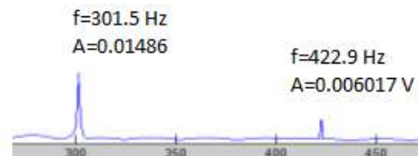
Figure 5. Frequency spectrum of the source voltage with load OFF, zoomed-in version.
